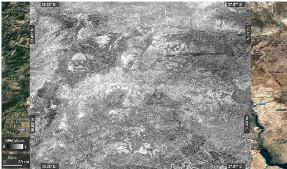
Figure 1. Damage proxy maps (DPM) generated by the AIRA team (ARIA Data Share 2023a) after the M7.8 Turkey–Syria earthquake, covering the area between 36^{\circ}62'E to 37^{\circ}87'E longitude and 36^{\circ}64'N to 37^{\circ}66'N latitude. The grayscale gradient indicates the level of detected damage, where a value of 0 represents no damage and a value of 1 indicates maximum damage. A scale bar in the lower left corresponds to 20 km, aiding in the estimation of affected areas' extents.
